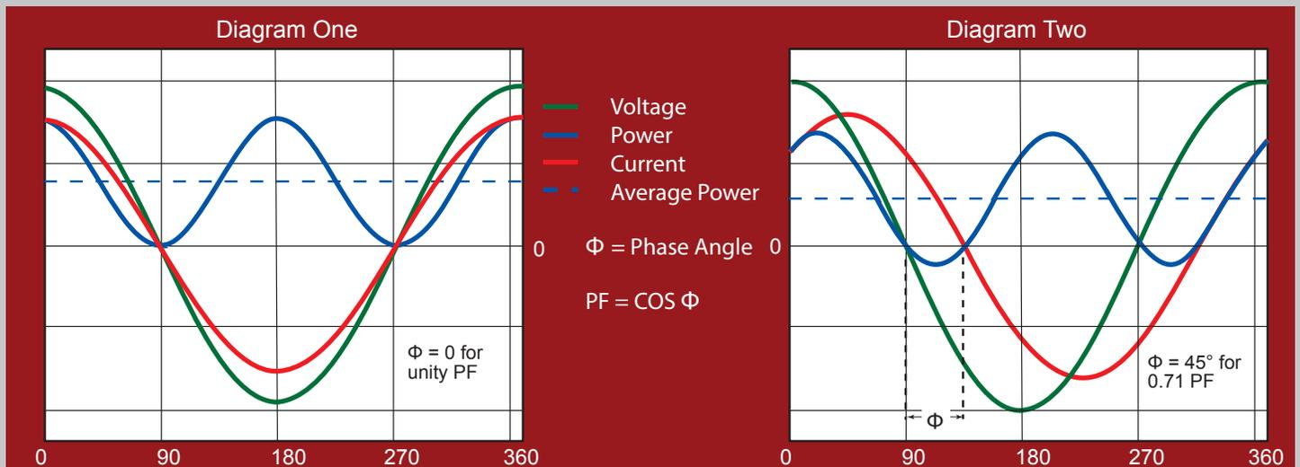
Purely resistive load connected with volts and amps in step for an unity (1) power factor when all the source energy is transferred and available to the load. Good power factors are normally greater than 0.9 to 0.95.
