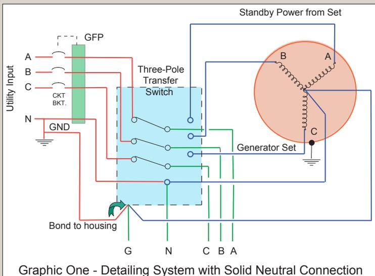
**Summary:** The general rule is when you have a grounded neutral at both the generator and the utility, you must use a transfer switch with enough poles to switch the neutral.
